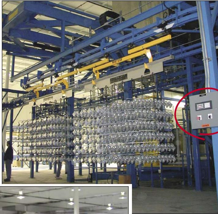
The Programmable Logic Controller (PLC) with racked parts in the background. The control panel is used by operators to enter recipes for various parts and substrates.
