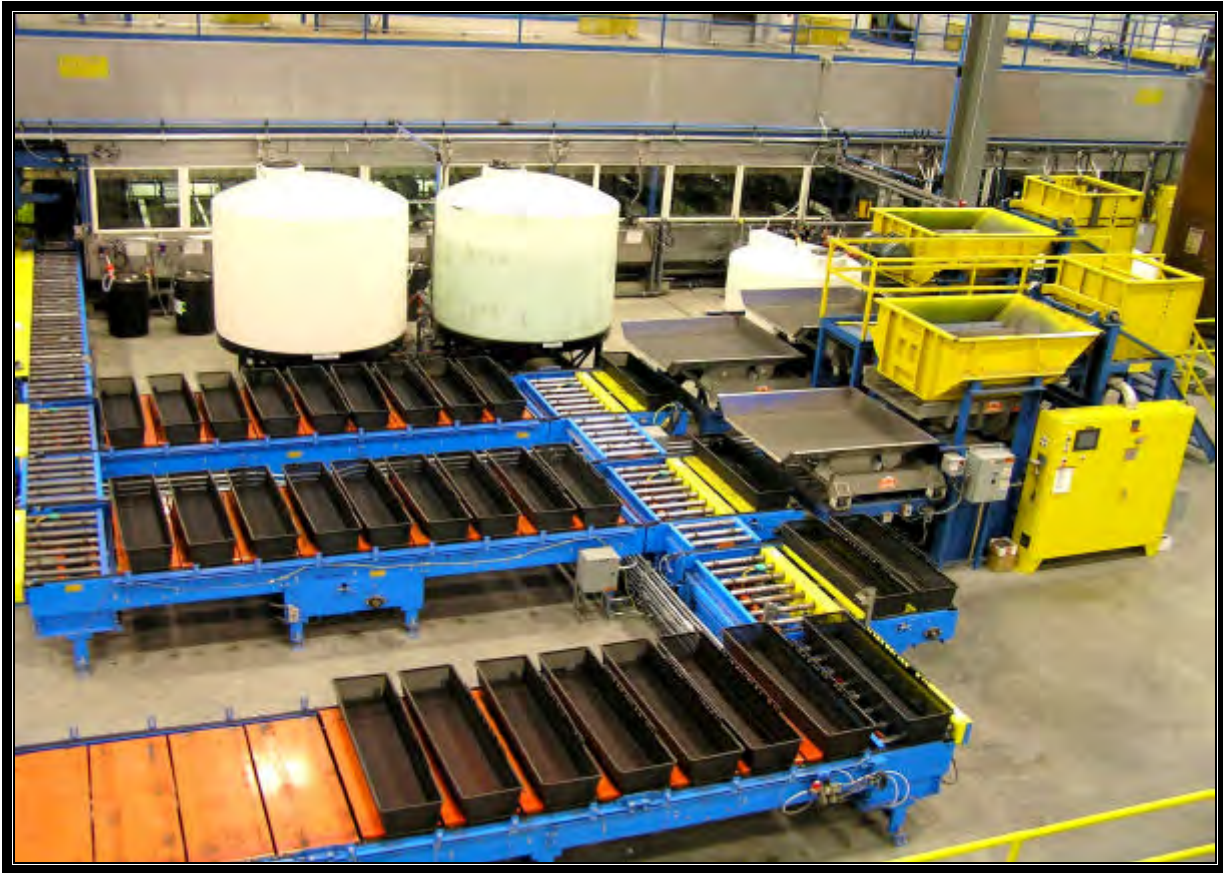
Figure 6. Live bottom hoppers and shaker tables measure fasteners into baskets by weight to prevent overloading.
