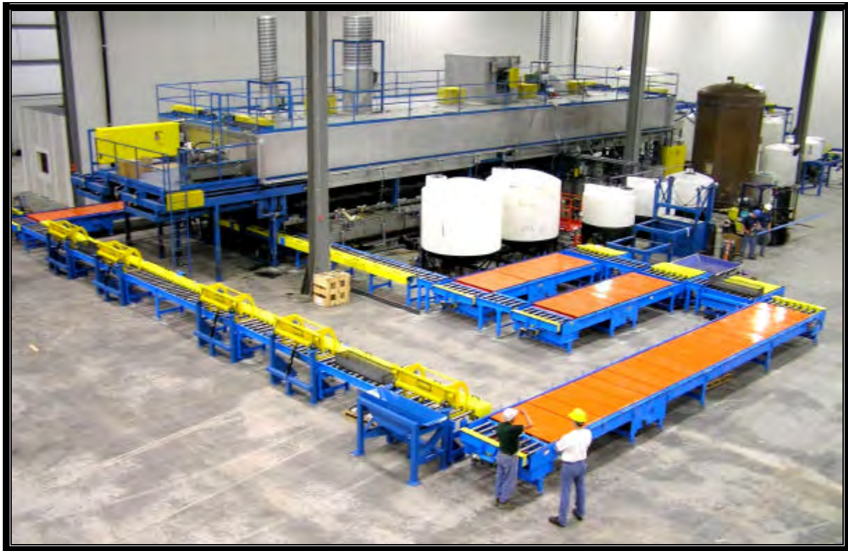
Figure 8. Five color square transfer electrocoating system with automated basket load/unload conveyor loop.
