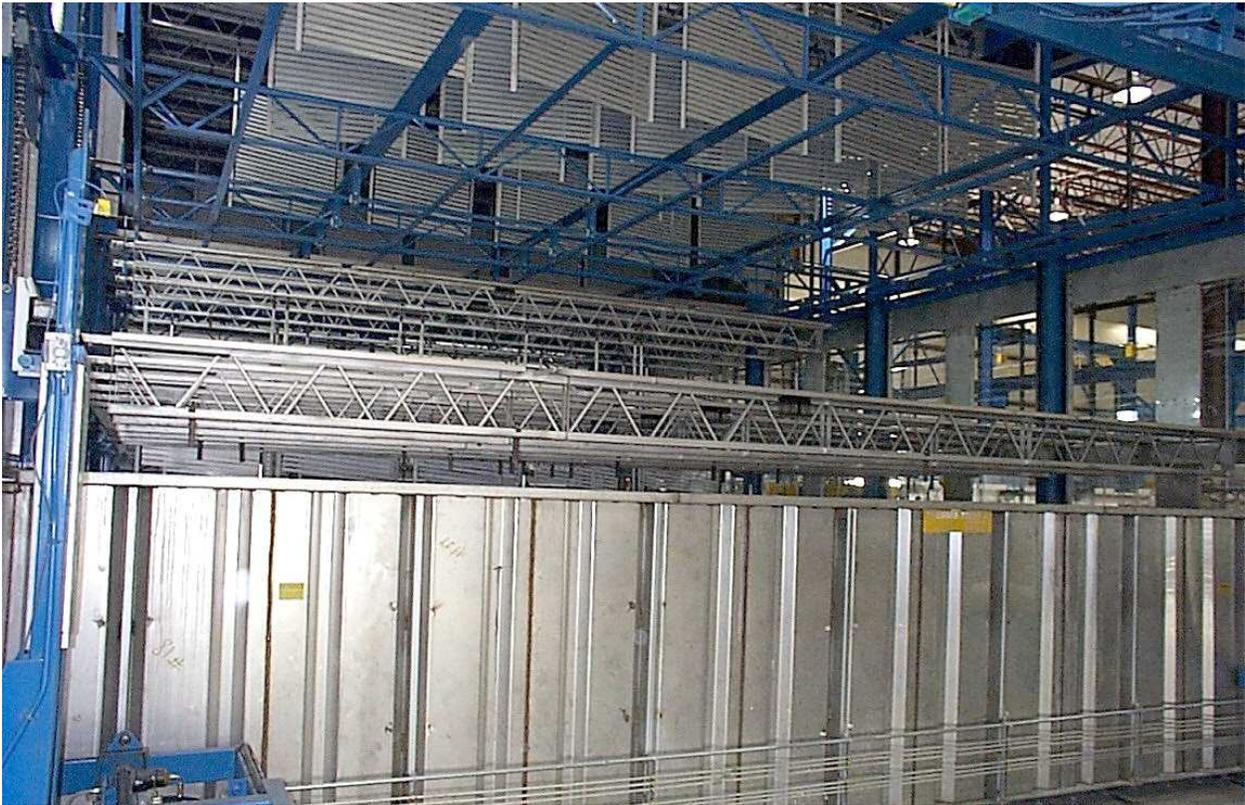
**Figure 3.** *In this powder coating system, aluminum parts undergo immersion pretreatment and dryoff in an indexing square transfer system (shown). Loadbars are then transferred to a power and free conveyor for powder application.*
