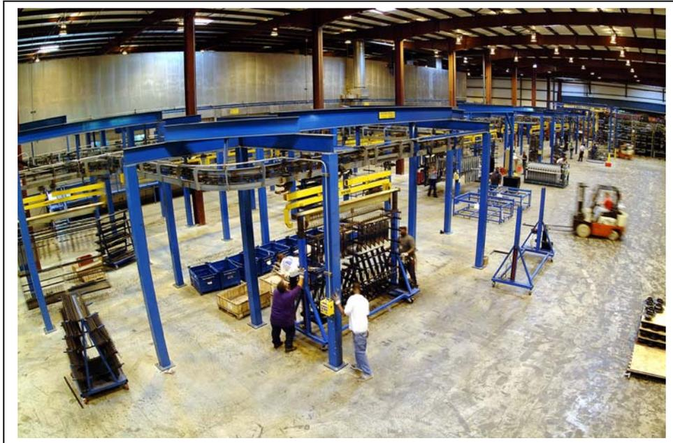
Figure 8: Power and Free Conveyor Load/Unload
