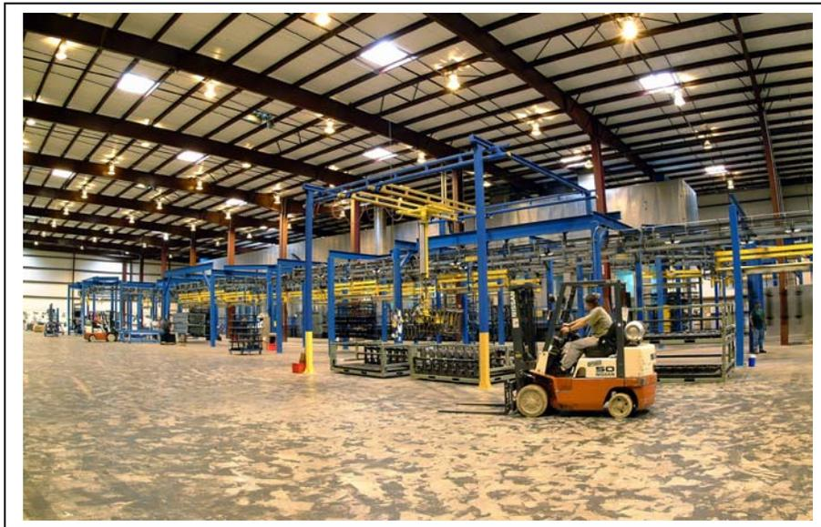
Figure 5: Power & Free Conveyor System
