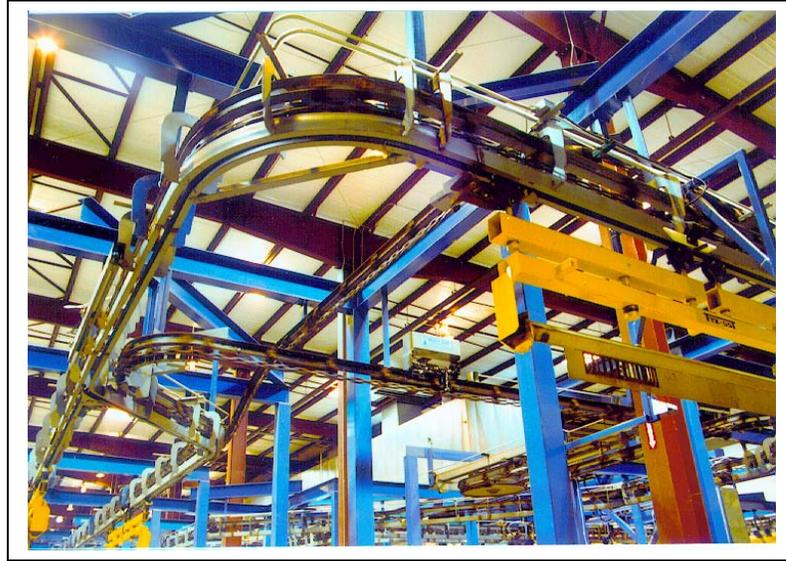
Figure 7: Power and Free Conveyor System
